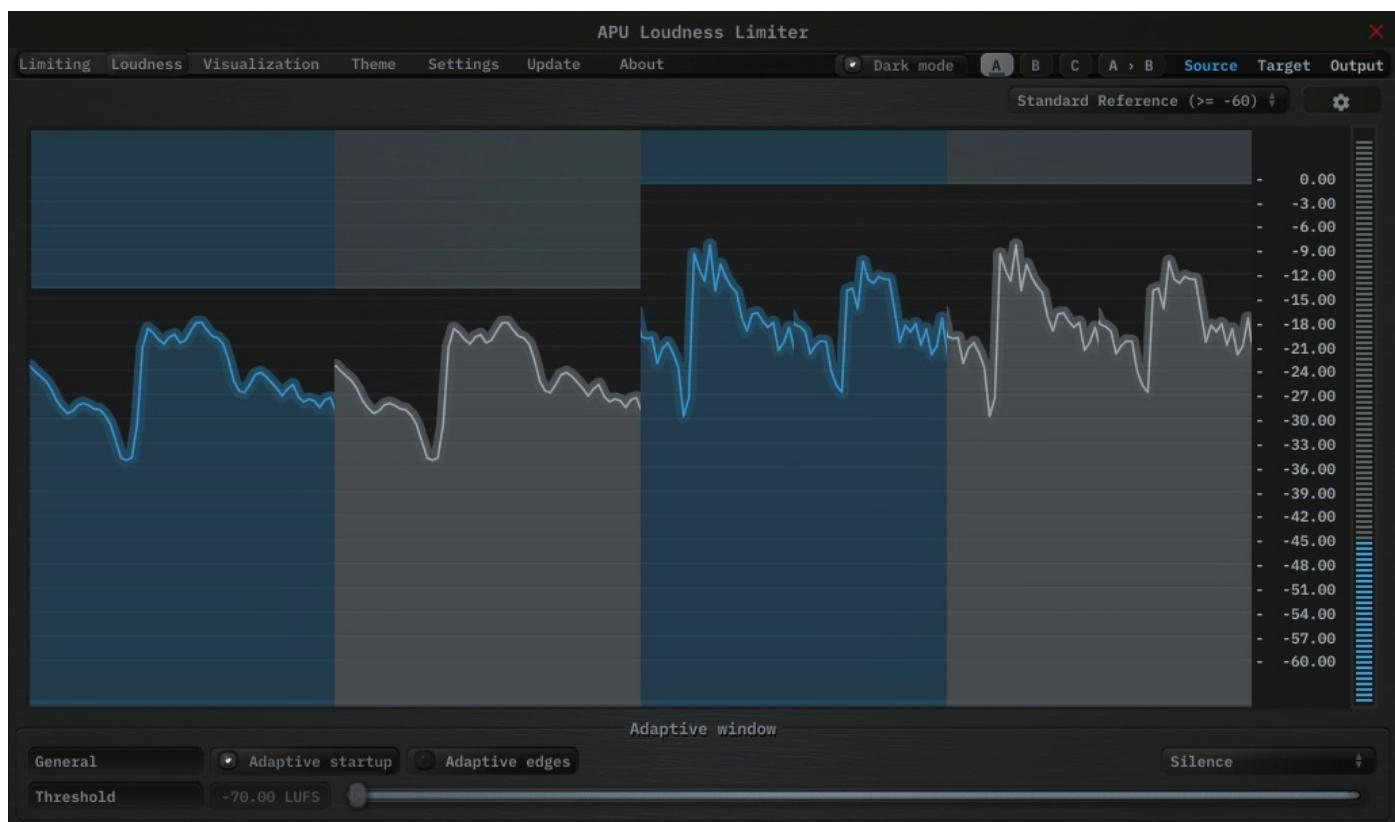
The loudness tab contains parameters relating to loudness measurements. You can configure adaptive window behavior here, which can be used to reduce transient artifacts during compression.
